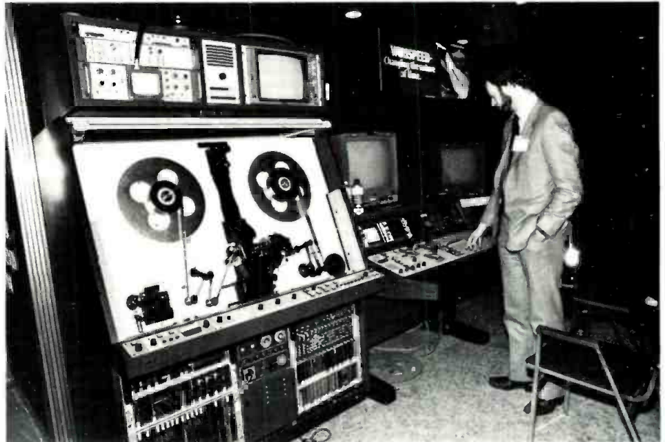
Rank Cintel's NAB exhibit featured the Mark IIC's new Varispeed capability, useful for slow motion and fast speeds as well as 30 fps transfer. Other telecine makers also promoted variable speed features.
