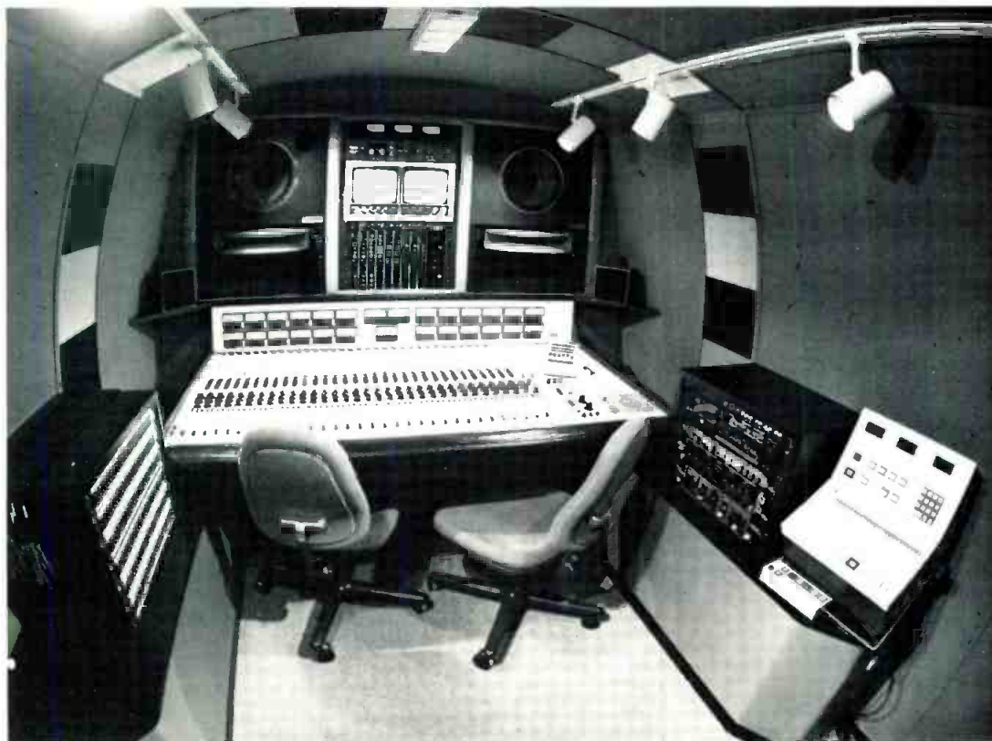
The Full Sail Dream Machine features a 32-input Sphere audio console. Fostex speakers are floated to avoid bass buildup; fabric walls help absorb sound reflections.
